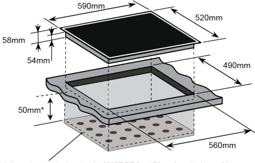
\* A thermal protection heat barrier MUST BE fitted 50mm from the base of the cooktop when access is possible via a cupboard or drawer. This thermal protection heat barrier should contain holes to improve ventilation as shown.
