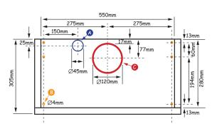
A Hole x 1 = position and size (45mm dia.) in shelf above rangehood for power cord
